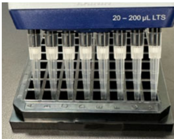
Figure 2: Pipetting into a well along the side wall.
